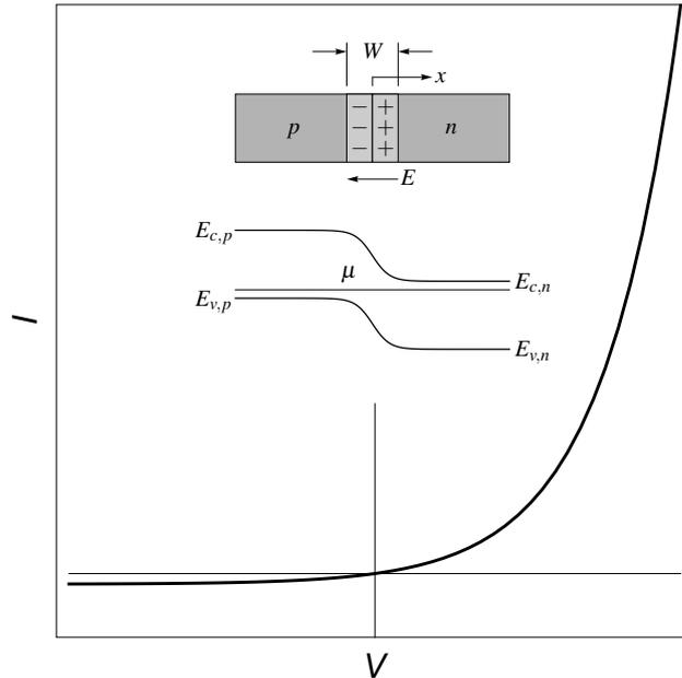
Current-voltage diagram showing the rectification properties of a  $p$ - $n$  junction, with a dramatic increase of current for forward bias ( $V > 0$ ), but only a small current for reverse bias ( $V < 0$ ). The inset shows a  $p$ - $n$  junction, along with the profiles of the valence and conduction band edges, and the important parameters that characterize the junction.
